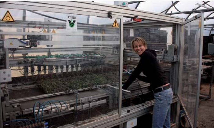
We use high speed machines to transplant tuberous begonias from small cells to larger cells.
