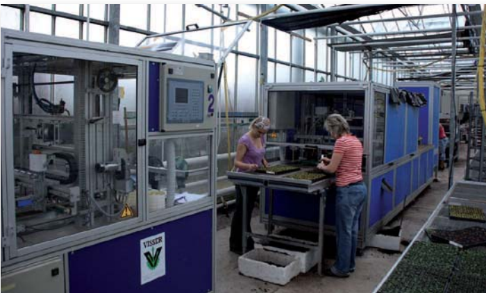
Replugging – All our trays are gapped before dispatch. We use our replugging machines to ensure each tray is 100% full, essential if you use transplanting machines.
